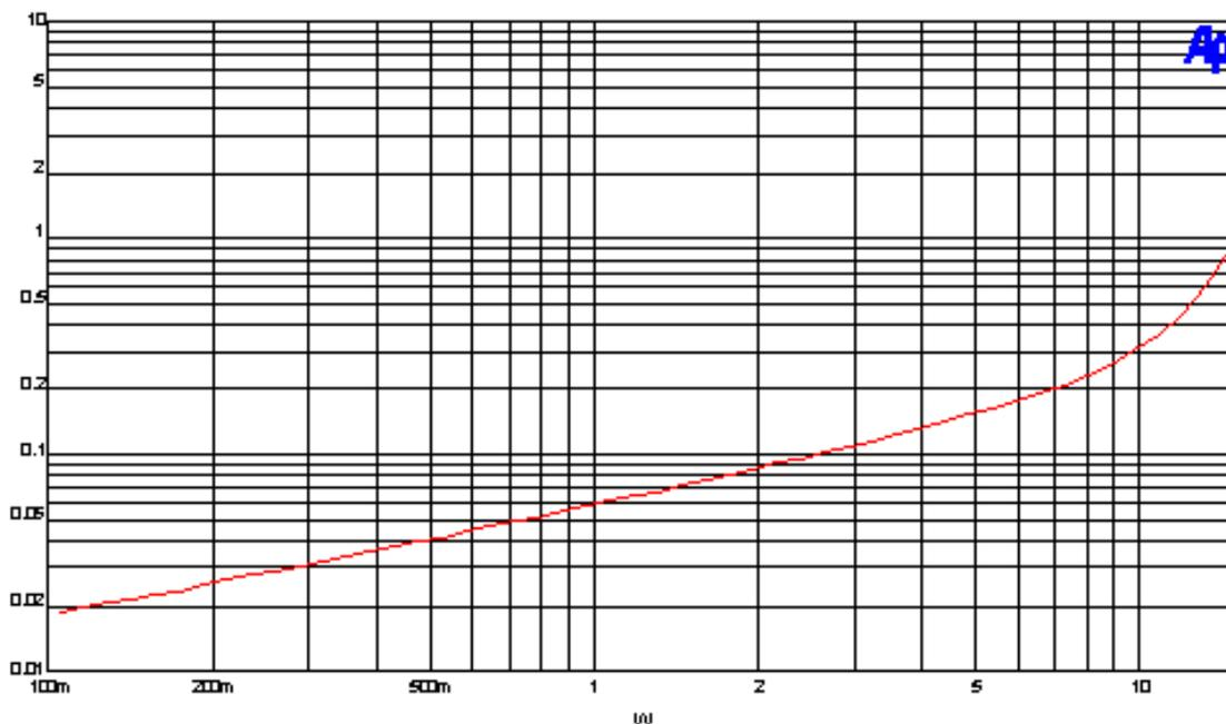
**Here's the distortion into 4 ohms at 1 KHz**
