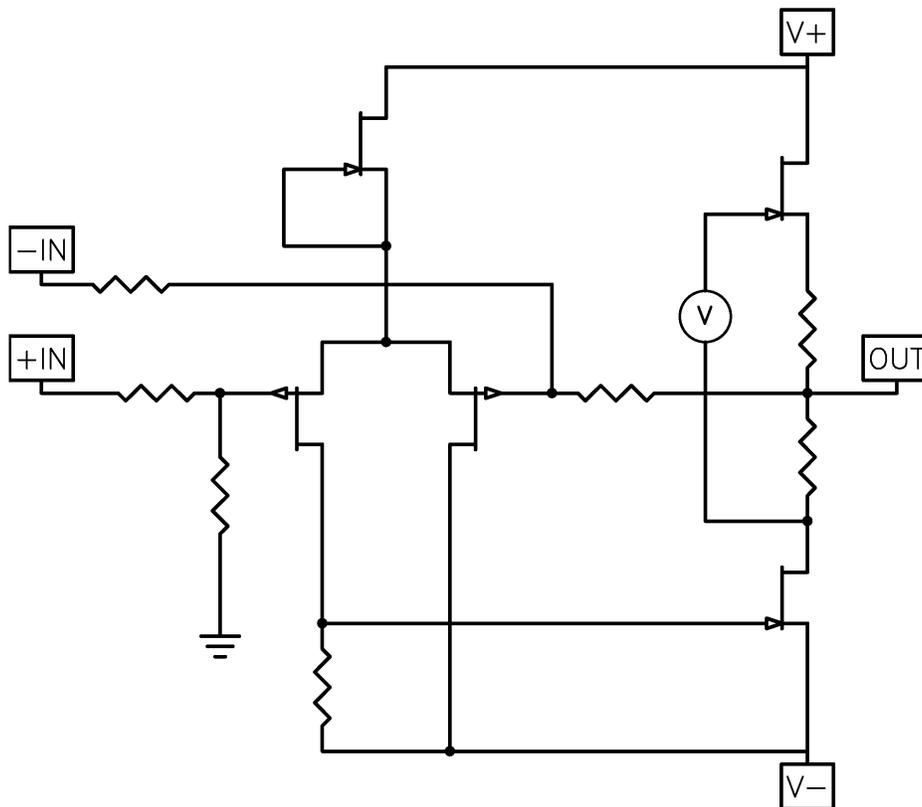
The most important topological difference is that the output stage current source is no longer an “Aleph” current source, but a version of the classic “Mu Follower”. This approach was chosen because the JFETs can take better advantage of distortion cancellation than Mosfets, but won't do so if the current source is tightly regulated. This has a little less precision, but lower distortion.
