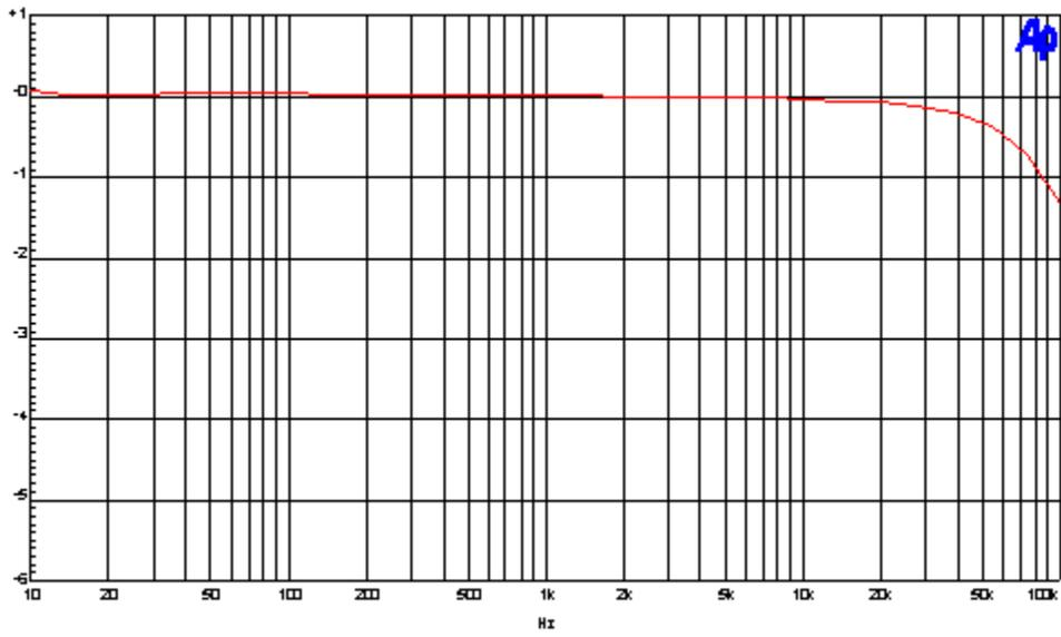
Here's the frequency response from 10 to 100 KHz
