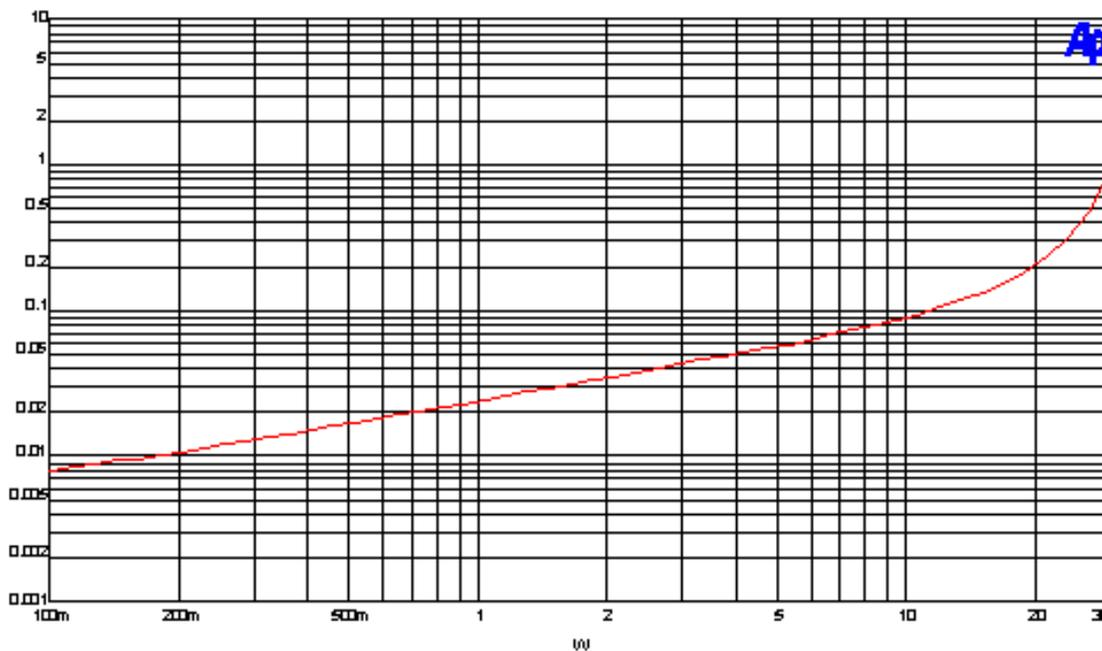
**Here's the distortion into 8 ohms at 1 KHz from 0.1 watts to 30 watts**
