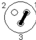
The XLR balanced input has pin 1 = ground, pin 2 = (+), and pin 3 = (-).
