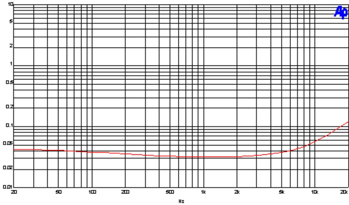
Here's the distortion into 8 ohms at 1 watt from 20 to 20 KHz
