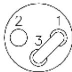
**Output Connection** - You can hook this amplifier up to any normal loudspeaker without danger of damage. Note, however that both the (+) Red output connection and the (-) Black output connection are live – neither is to be treated as if it were ground. This can be important when you are hooking up active sub-woofers to the output of the amp – if you need a ground connection then use the white ground terminal provided on the rear panel.
